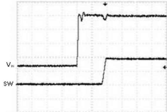
Start-up from Shutdown (1V/DIV 100ns/DIV)
